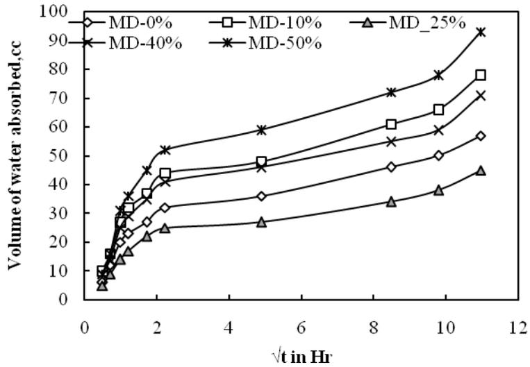
Figure 10: Water absorption of Mortar cubes with Marble powder
