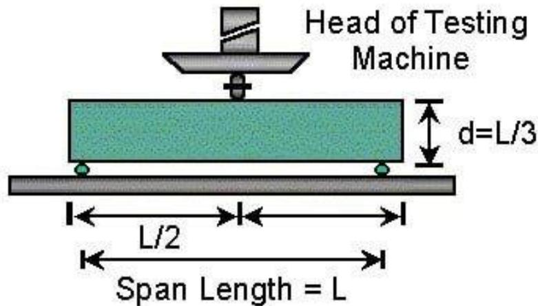
Figure 5: Schematic representation of flexural testing
