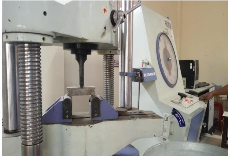
Figure 6: Testing of the mortar specimen under flexure
