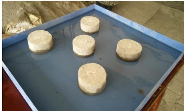
Figure 8: Mortar cube with marble powder under water absorption
