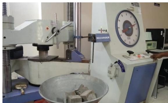
**Figure 3: Testing of the specimens under compression**
