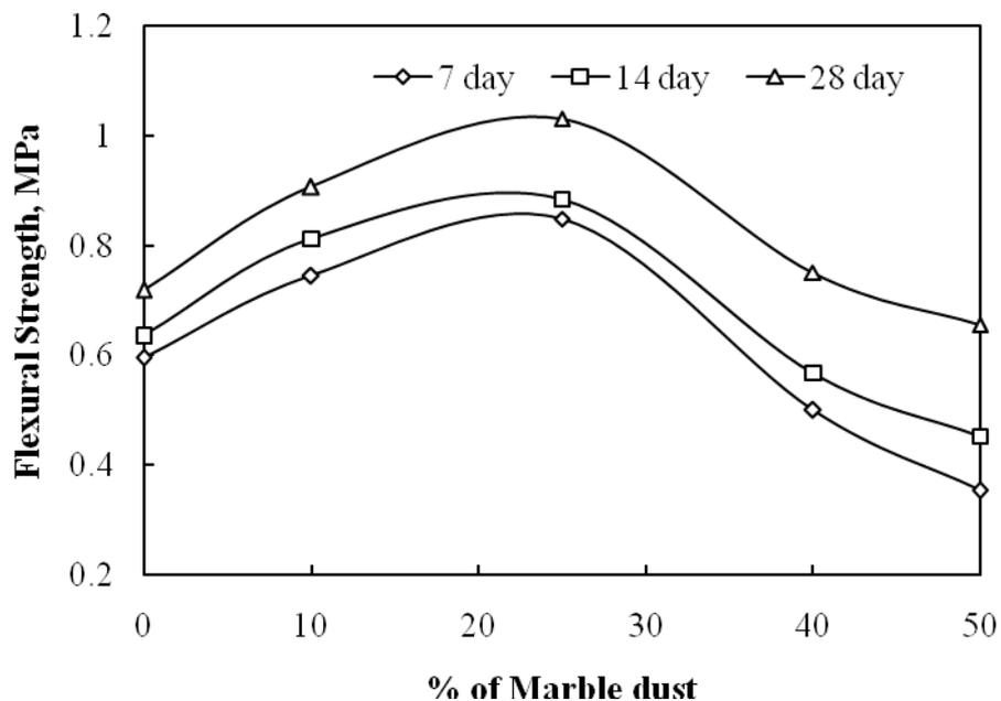
Figure 7: Flexural Strength of the Marble replaced mortar cube
