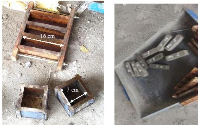
**Figure 2: Fabrication of mould and casting of specimens**
