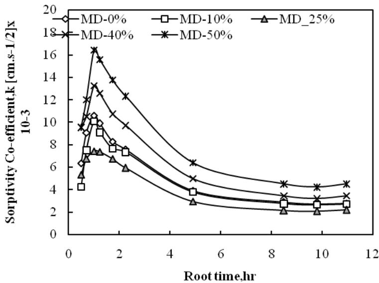
Figure 11: Sorptivity Coefficient of Mortar cubes with Marble powder
