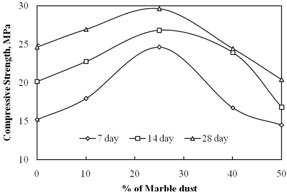
Figure 4: Influence of marble dust in compressive strength of mortar cube
