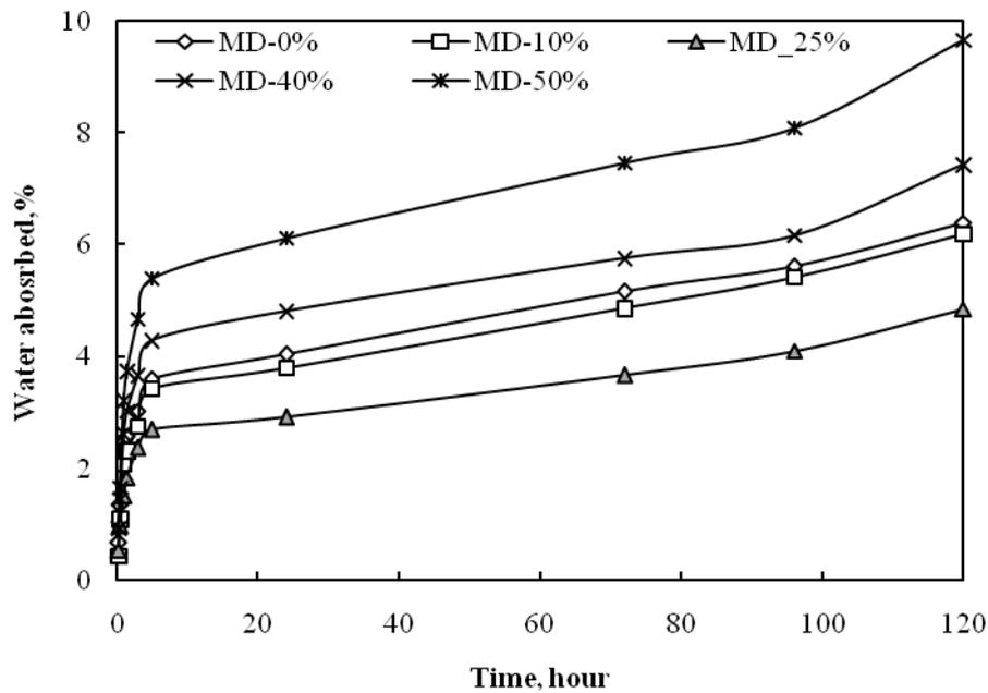
Figure 9: Rate of water absorption versus Time for the test samples
